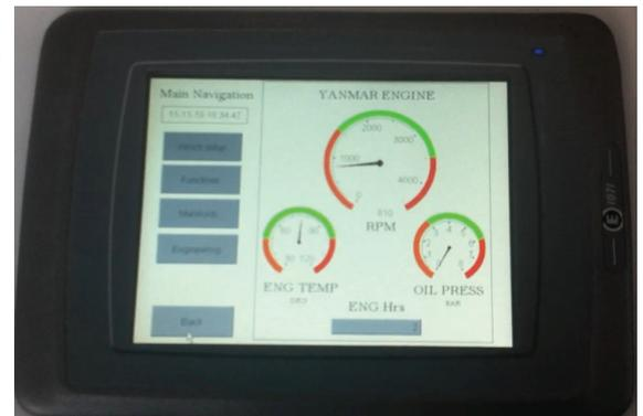
The PLC plays an important roll not only controlling the hydraulics, but also taking complete control of the engine functions. The yacht has two electronic throttles at port and starboard helm positions that are fully integrated to the PLC. Engine monitoring is also performed on the E1000 series HMI this removes the traditional engine gauge panel helping to reduce weight!
