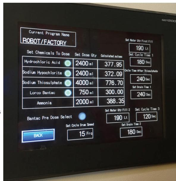
Above, the inside touch screen display currently showing a recipe setup page. All touch screen pages are designed bespoke for the application and convey complex detailed information in a from that is clear, and simple to follow.
